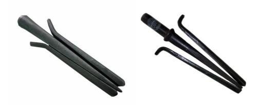
Wedges (Plugs) and feathers are also known as Wedge and Shims or Wedges and Feathers, they are among the oldest styled tools still used today and remain one of the best methods of splitting stone, these tools designed to split rock when driven into a drilled hole or natural crack. The wedge fits in the hole between two feathers whose flat side form a guide that prevents the wedge from jamming as it is driven into the hole.
